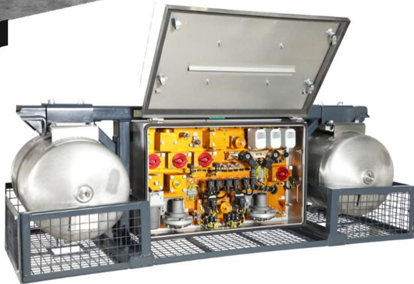
**Description :** The brake module supplies the output pressure (BC) through a main relay valve which is piloted by an electro-pneumatic circuitry (magnet valves and pressure transducer operated in closed loop by the BCE).
