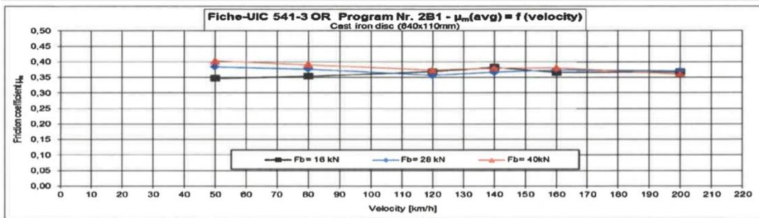
Typical friction coefficients for axle mounted discs according to UIC program 6A. The tested pad was the SF140FF/350.
