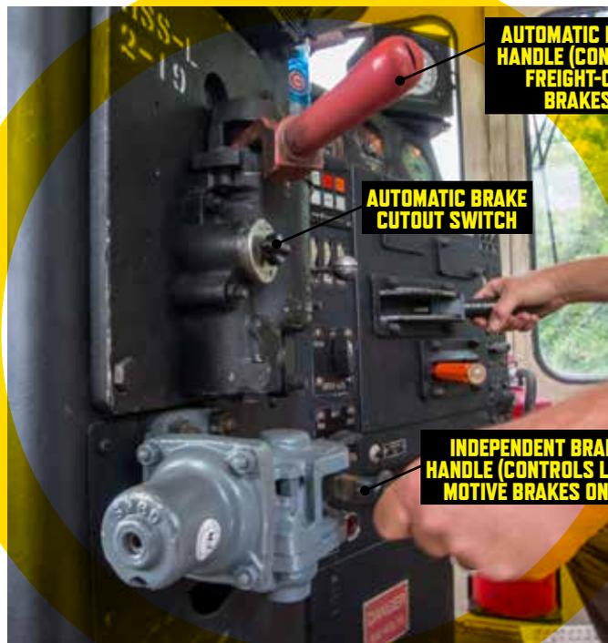
● Parts of the air-brake system: Air gauges, levers, and switches, aboard Burlington Junction MK1500D No. 9630, along with the engineer work together to stop the train. Two photos, Steve Smedley
