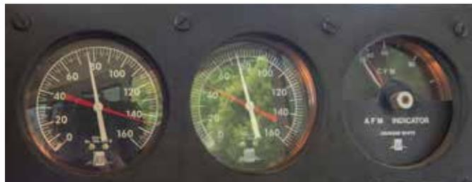
● **LEFT GAUGE** Red: main reservoir pressure, White: equalizing reservoir pressure. **MIDDLE GAUGE** Red: brake-cylinder pressure (locomotive), White: brake-pipe pressure (locomotive and cars). **RIGHT GAUGE** Air-flow indicator (not on all locomotives).
