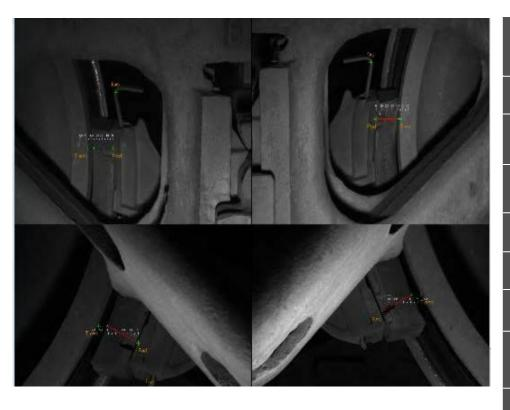
Brake pads on trains are designed to wear. The composite brake pad is designed to provide friction between the wheel tread and the brake pad (shoe), but the wear rate of the brake is much greater than that of the wheel so that the inexpensive brake wears out before the expensive wheel.
