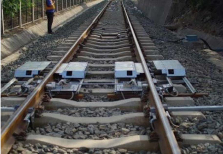
Wheel management is of key importance to cost-effective rolling stock maintenance. Wheels are among the more expensive items to maintain and replace. The Track IQ Wheel Profile Monitor (WPM) is a track mounted machine vision system that not only measures individual wheel parameters but also performs measurements on the entire wheelset for each axle of the train.
