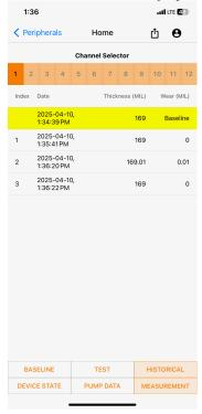
c. The baseline reference will be displayed in a yellow bar, with the subsequent readings (or thickness) displayed below. Each reading will have the date and time it was taken, and its variance to the baseline in mils. This will enable you to quickly scan for any wear trends. Variances within +/- 0.3 mils are within the accuracy range of the system and do **not** indicate any wear on the bearing.
