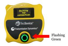
e. The reader should now be listed in the App. Each reader will have a unique address code. If no devices are shown, make sure the Bluetooth Status is "On". If your Bluetooth is "Off", shut down the app, turn on your Bluetooth, and restart. When the reader is shown on the list, tap on its listing.
