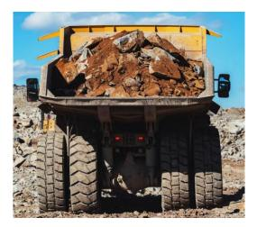
The Truck Particle Size Analyzer, PSA, system is a reliable and robust machine vision-based system from Wabtec Digital Mine and Stone Three used to measure the size distribution of bulk material such as mineral ore on haul trucks. This system makes use of the latest industrial high-resolution and wide dynamic range camera technology for superior accuracy and robustness.
