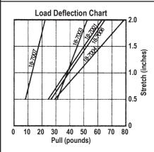
Determine stretch or holding force required from load deflection chart and add zero-stretch dimension A or B to locate hood bracket in relation to anchor bracket.
