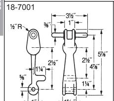
With anti-rattle nub. Our standard model. Especially suited to fastening truck hoods and for heavy-duty applications.
