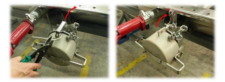
Rotate the nozzle cap counterclockwise until it hits the stops. Once it hits the stops, pull the cap towards you to remove. The vacuum unloading hose can now be attached to the gate. Do NOT power up the vacuum pumps on the unloading system yet.
