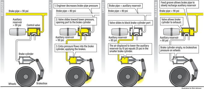
the brakes. The second was a triple valve to control the three states of the braking system: charge, apply, and release. One was mounted on each car, and it controlled the system by being connected to the brake pipe, auxiliary reservoir, and brake cylinder.
