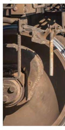
a 1% grade, exerted in excess of 7,600 hp worth of stopping power, and dissipating the energy as heat in the brakeshoes and wheels. From 20 mph, the train could be stopped in 176 feet.
