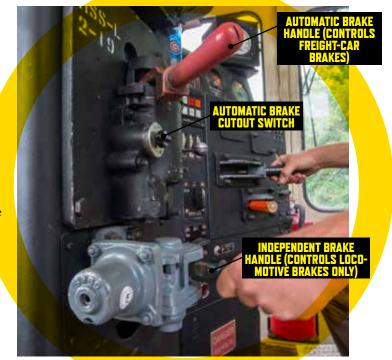
Parts of the air-brake system: Air gauges, levers, and switches, aboard Burlington Junction MK1500D No. 9630, along with the engineer work together to stop the train. Two photos, Steve Smedley
