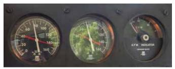
• LEFT GAUGE Red: main reservoir pressure, White: equalizing reservoir pressure. MIDDLE GAUGE Red: brake-cylinder pressure (locomotive), White: brake-pipe pressure (locomotive and cars).
