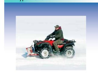
In almost every plowing application Longwood rubber snowplow blades make the best kind of sense. They are flexible – so they conform easily to road surfaces for clean snow removal. They won't gouge road surfaces. They operate smoothly on high-speed runs. They won't tear up or damage raised reflective pavement markers.
