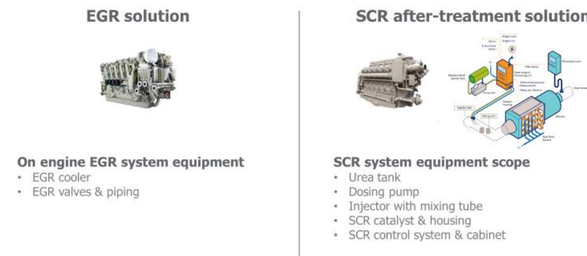
Figure 2. Difference in equipment scope for EGR and SCR technology
