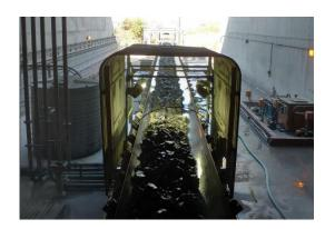
A Digital Mine solution offering from Stone Three and Wabtec's Digital Mine offers its latest deep learning Particle Size Analyzer (PSA) to help improve accuracy. The PSA system is a reliable and robust machine vision-based system used to measure the size distribution of bulk material such as mineral ore on a conveyor belt. The PSA makes use of the latest industrial high-resolution laser and camera technology for superior accuracy and robustness.
