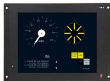
**Driver Machine Interface "DMI"** in a panel option or digital visual display unit on a single touchscreen
