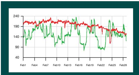
This graph shows the monthly natural gas usage from before the sensors were installed (red) and after Damon's team started using sensors to adjust furnaces (green). The old usage was very steady and consistently high, but the new usage varies as valves open and close to maintain a target temperature zone.
