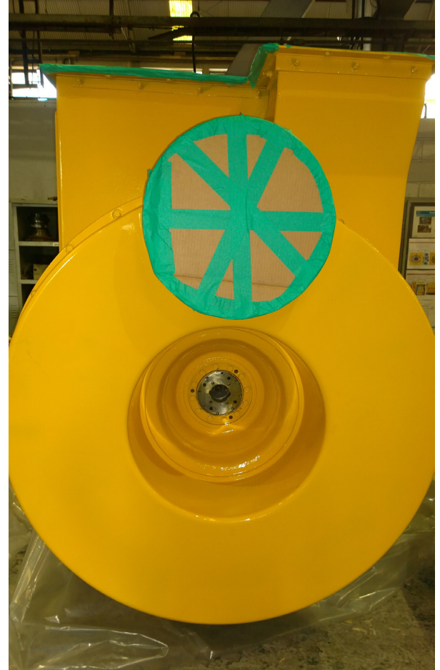
GTA41 traction alternator from a Komatsu mining truck, a key component that generates the electrical power needed to drive the truck's traction motors.
