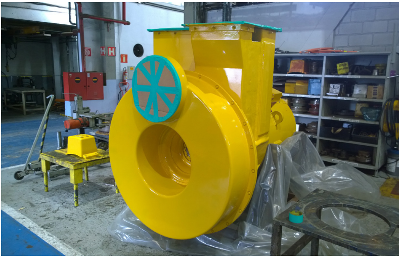
GTA41 traction alternator from a Komatsu mining truck, a key component that generates the electrical power needed to drive the truck's traction motors.
